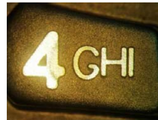
Figure 9: Multi pass 3X a t 500Khz, 10ns, 10W, 301000mm/s
